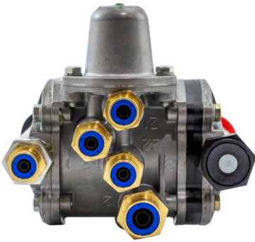
KNORR BREMSE PARK SHUNT VALVE
